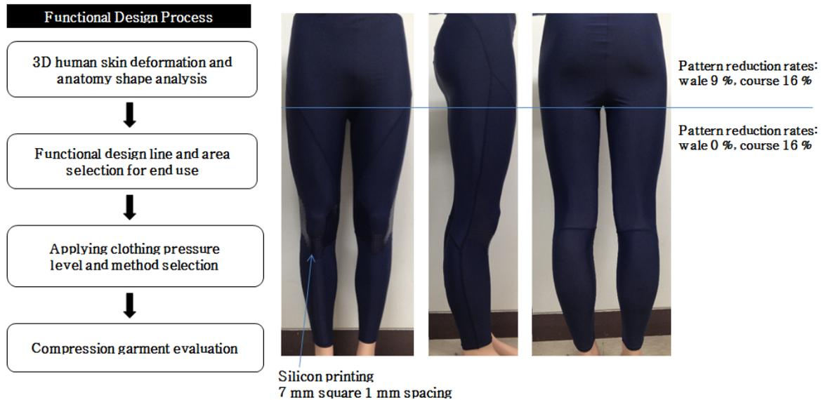
[Figure 8] Process and characteristics of the development 3D compression garment
