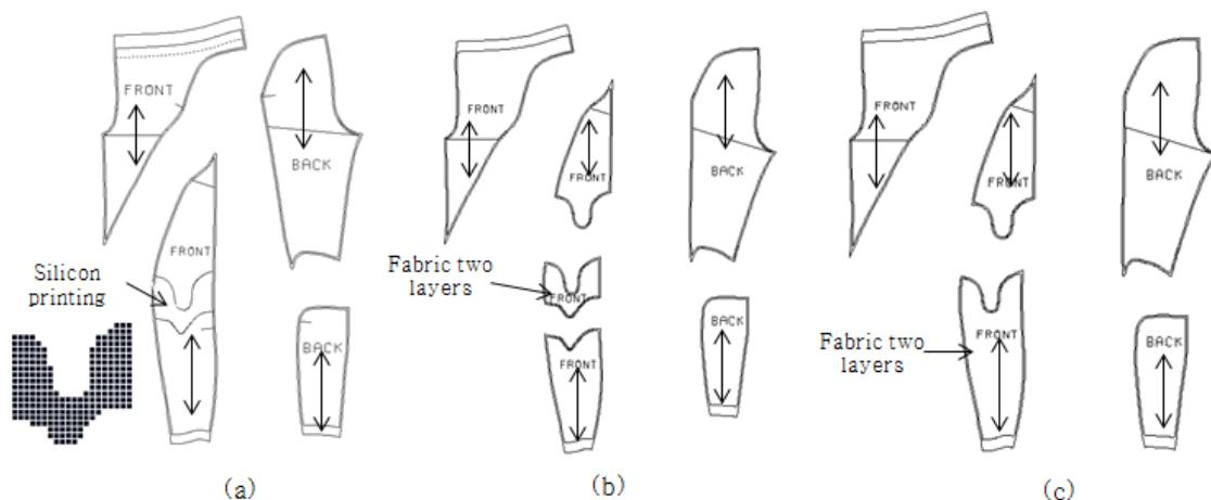
[Figure 7] Patterns for each 3D compression garment design
