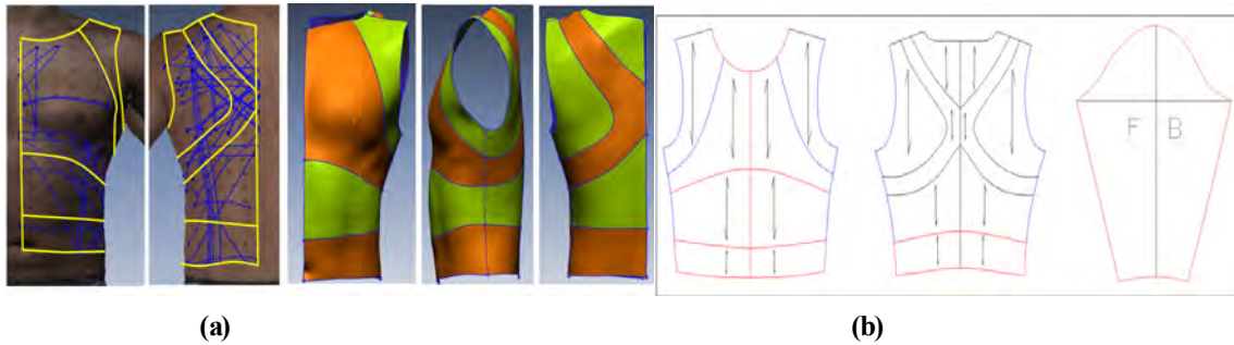
[Figure 12] Performance cutting line using the LoNE(a) and 3D-2D pattern(b)
