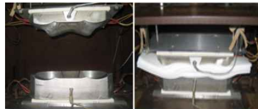
[Figure 4] Mold case and thermal forming for manufacturing of the mold brassiere cups
