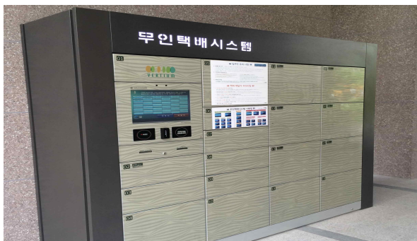
Figure 4. E apa.: Unmanned delivery system
